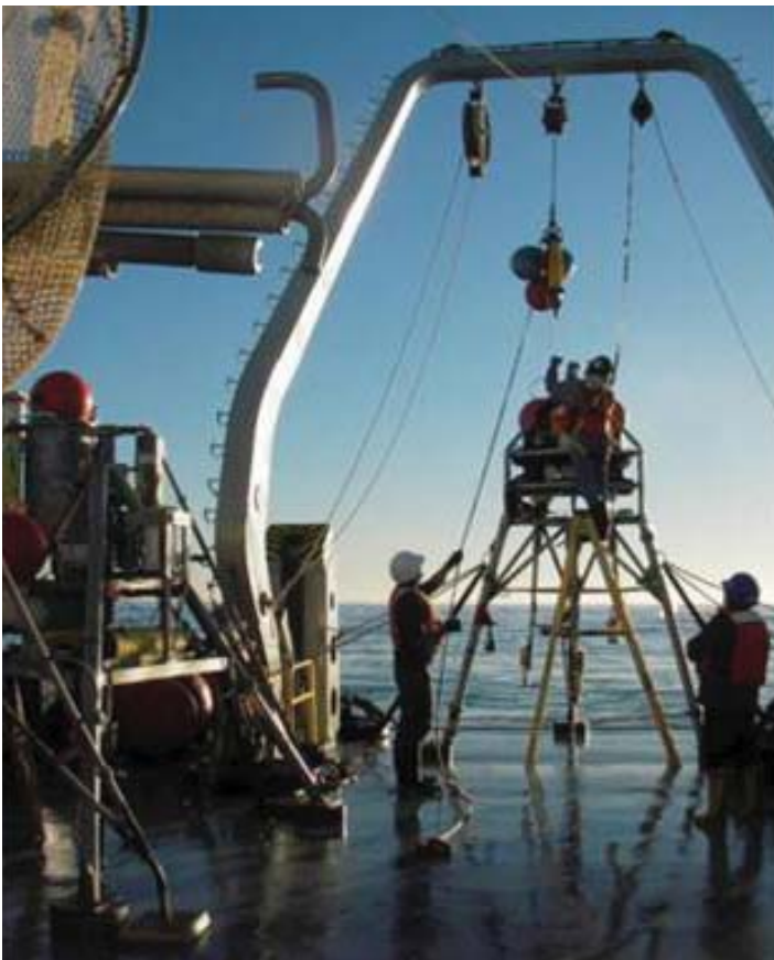
Figure 3: USGS placed tripods on the PV Shelf floor to collect data on winter storms
